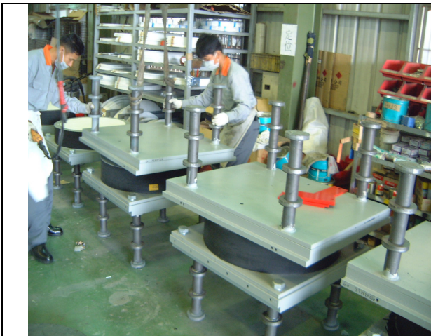
Fig. 16 – 17 Antivibrating bearings for the Taiwan High Speed Railway. Picture 16 shows the assembling phase in the factory; Fig. 17 the scheme. The lateral vertical steel plates shown in the scheme (not yet applied in Fig. 16) are anti-lifting devices
