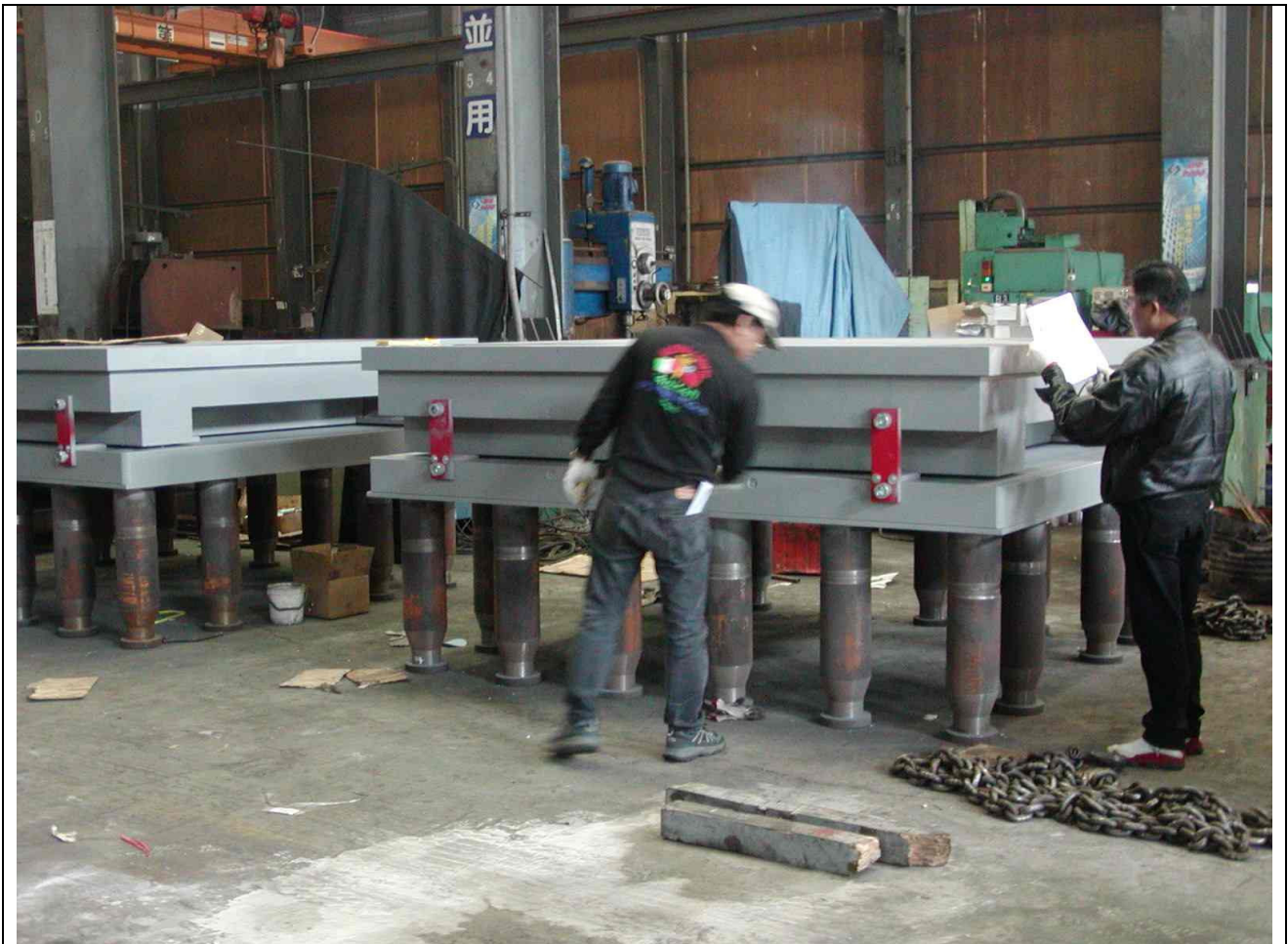
Fig. 15 – Giant shear key for the Taiwan High Speed railway. The red steel plates are intended for installation purpose only
