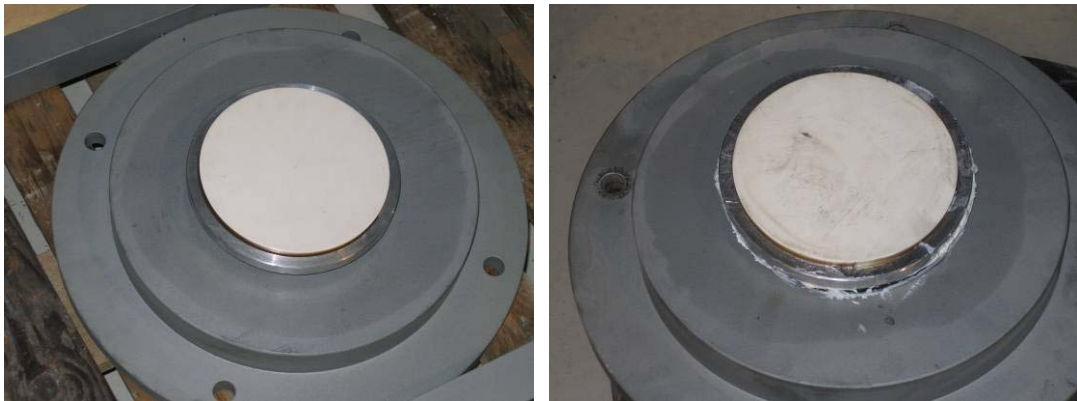
Figure 10 Comparison between the sliding surface before tests (left side) and at the end of test campaign (right side); no damage occurred and no evidence of deformation due to temperature effect due to the energy dissipation by friction.
