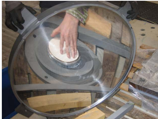
Figure 3 Sliding plate of the single surface sliding pendulum, the sliding surface is in stainless steel and appears like a mirror
