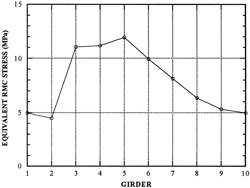
FIGURE 55.15 Equivalent stresses for girders in bridge U.S. 23/SR.
