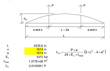
Find the Estimated Deflection at the Pier of the Bridge for a Two Point Load at Piers with Infinitely Stiff Abuts. In Terms of an Applied Load "P".
