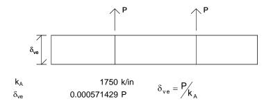
Find the Fraction of the Estimated Pier Deflection at the Piers Versus that at Center Span
