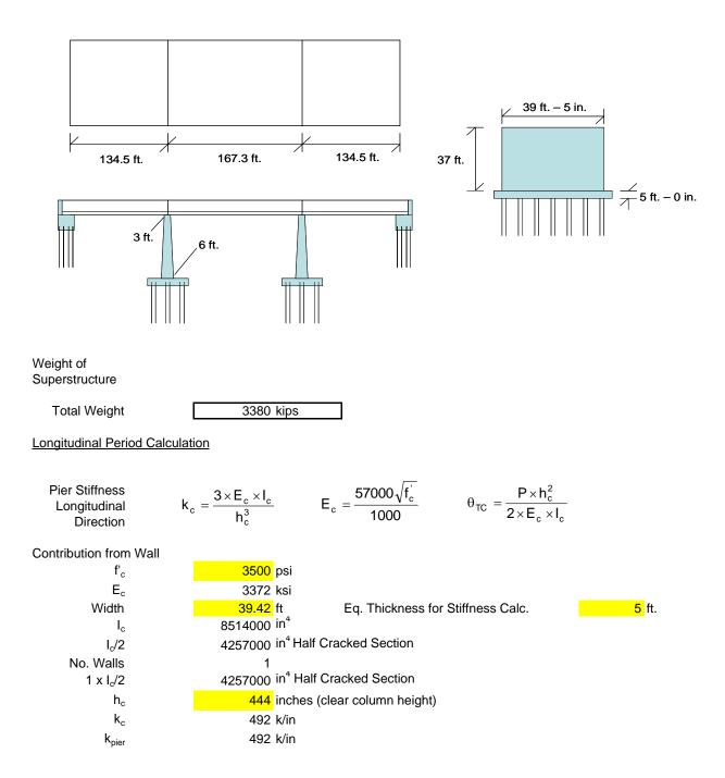
Long. Base Sh & Displ Pg. 2 Contribution from Cap Beam (Stiffness is infinite but it deflects as a rigid body and contributes to pier stiffness)
