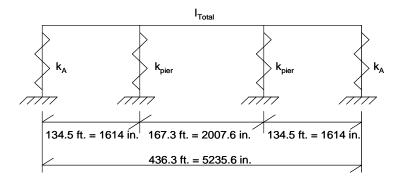
Estimate the Abutment Pile Transverse Stiffness k<sub>A</sub>
