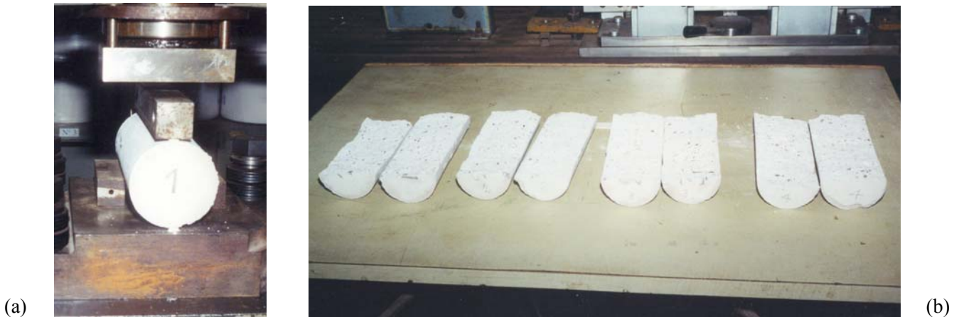
Fig. 2.2. Cylinder splitting (“Brazilian”) test. (a): Apparatus set; (b) Split specimens.
