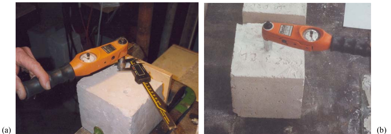
Fig. 3.2. (a): device expansion and calibre controlled reset; (b): torsional test.
