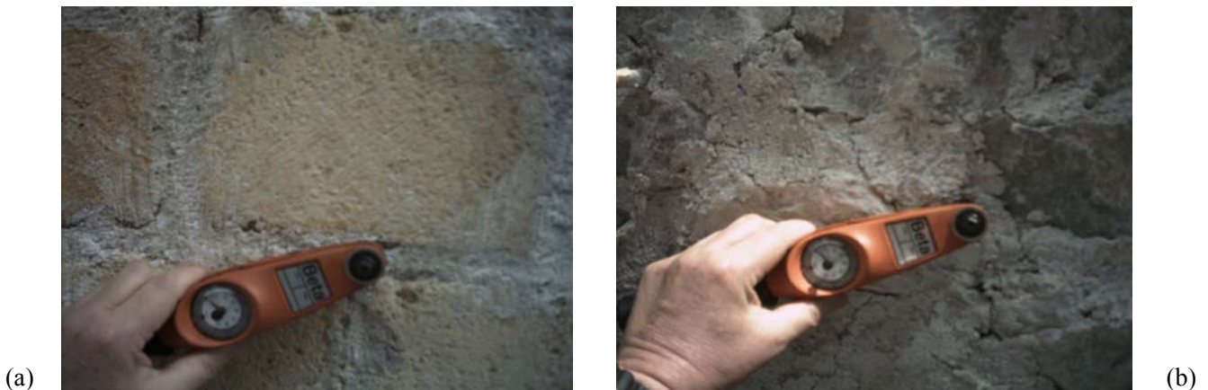
Fig. 3.2. In situ torsional tests on tuff masonry walls. (a): ashlar; (b): rubble course.
