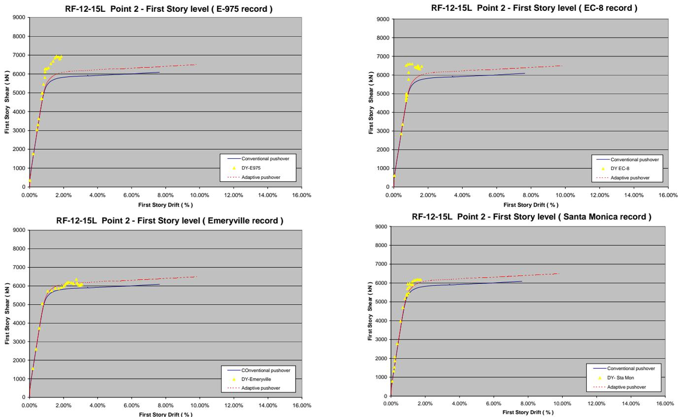
Figure 4.4 Response at the first story level, regular structure ( low ductility )
