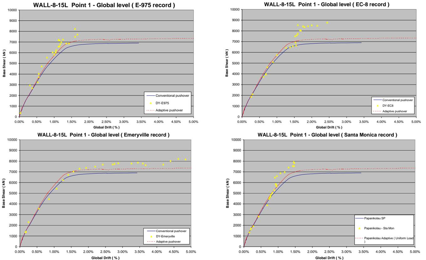
Figure 4.12 Response at the global level, frame-wall structure ( low ductility )
