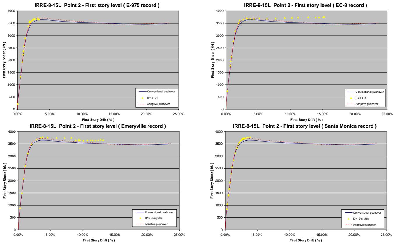
Figure 4.25 Response at the first story level, irregular structure ( low ductility )
