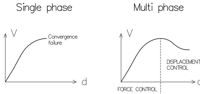
Figure 2.6 Single versus multi-phase solution
