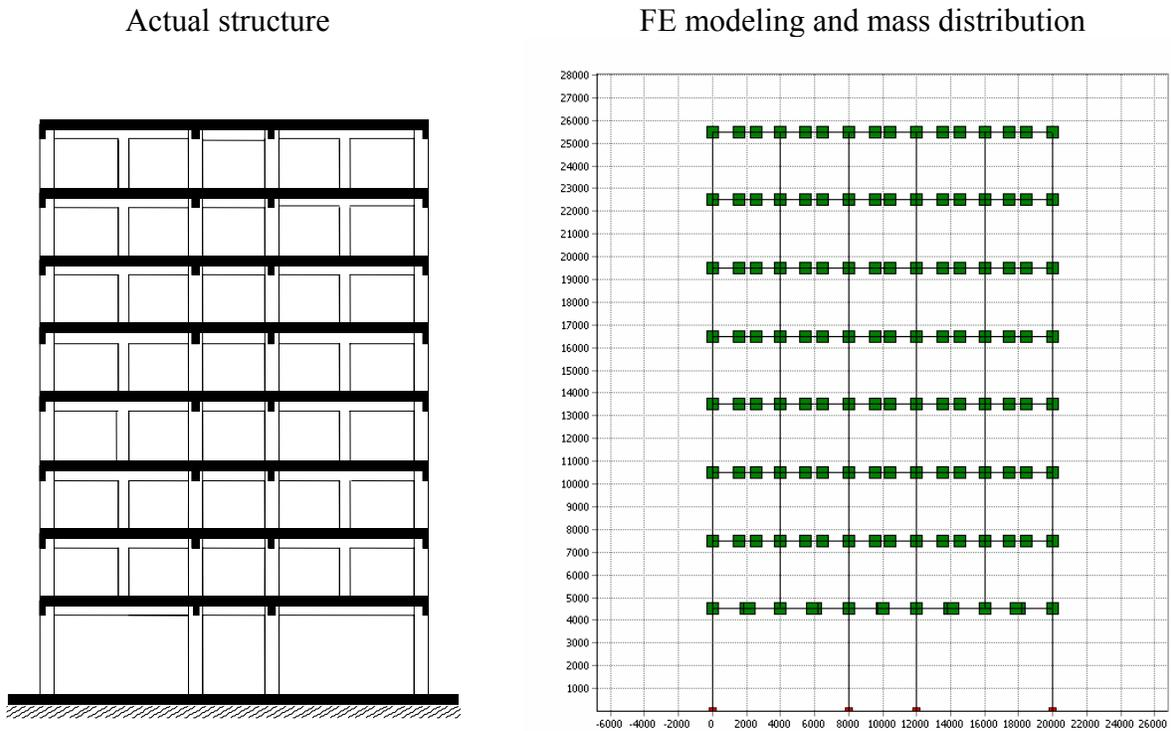
2D reinforced concrete frame
