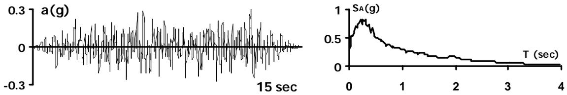
Figure 3.10 Scaled accelerogram and response spectrum of the E975 record
