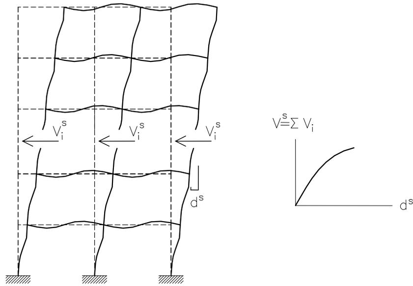
Figure 3.15 Story shear versus interstory drift monitoring
