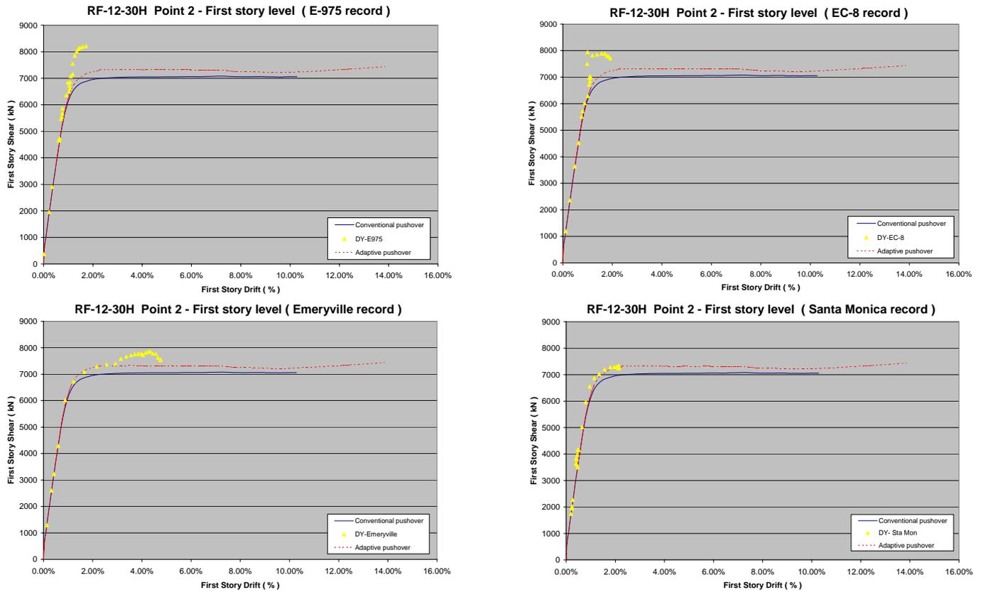
Figure 4.3 Response at the first story level, regular structure ( high ductility )
