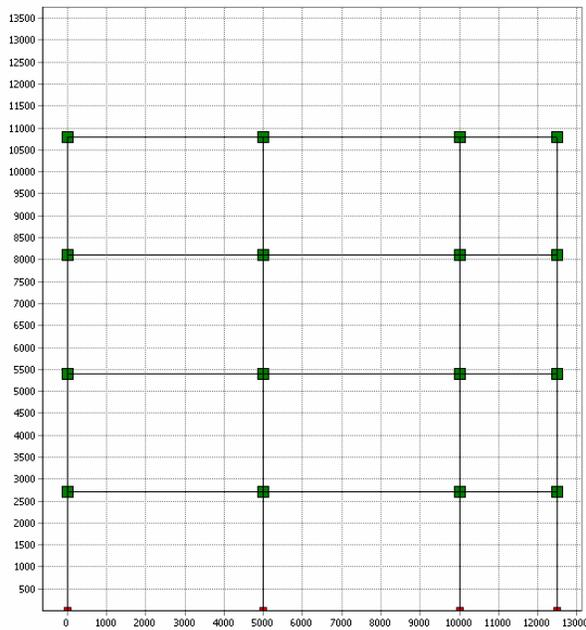
2D reinforced concrete frame
