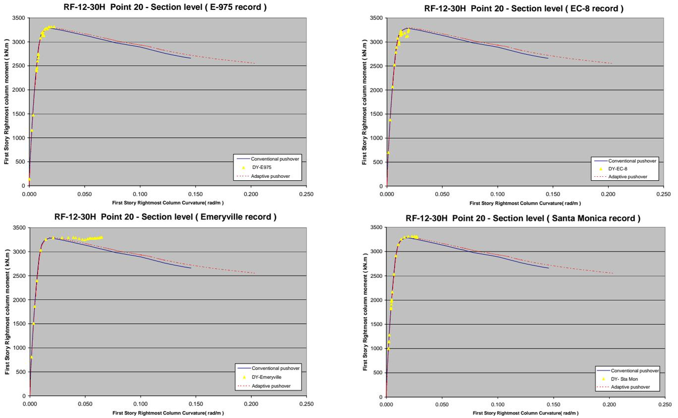
Figure 4.7 Response at the section level, regular structure ( high ductility )
