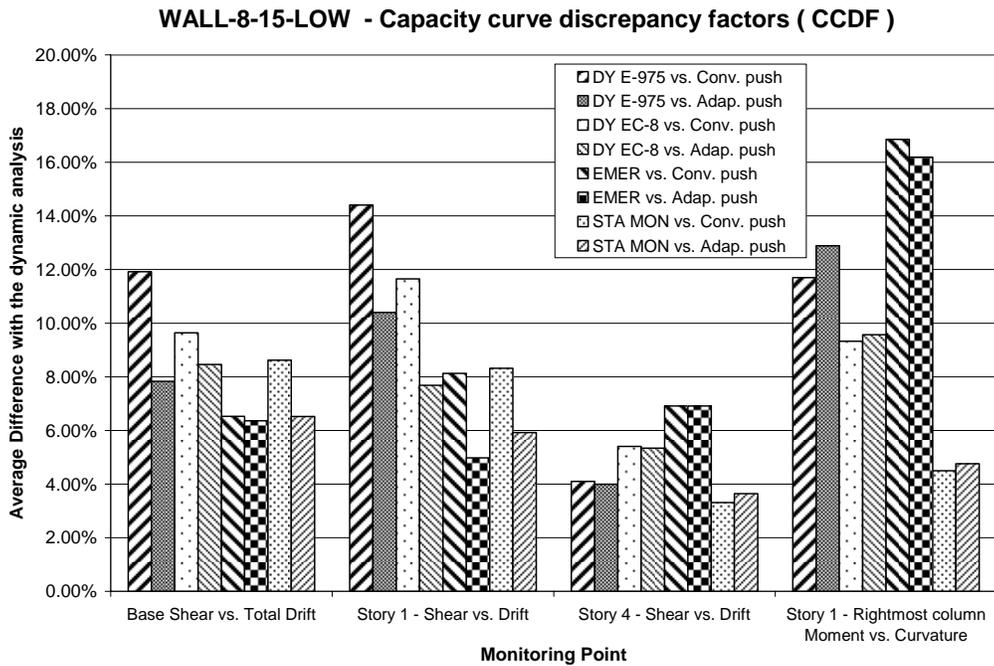
Figure 4.21 Results summary, frame-wall structure ( low ductility )
