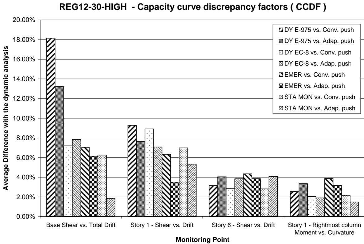
Figure 4.9 Results summary, regular structure ( high ductility )
