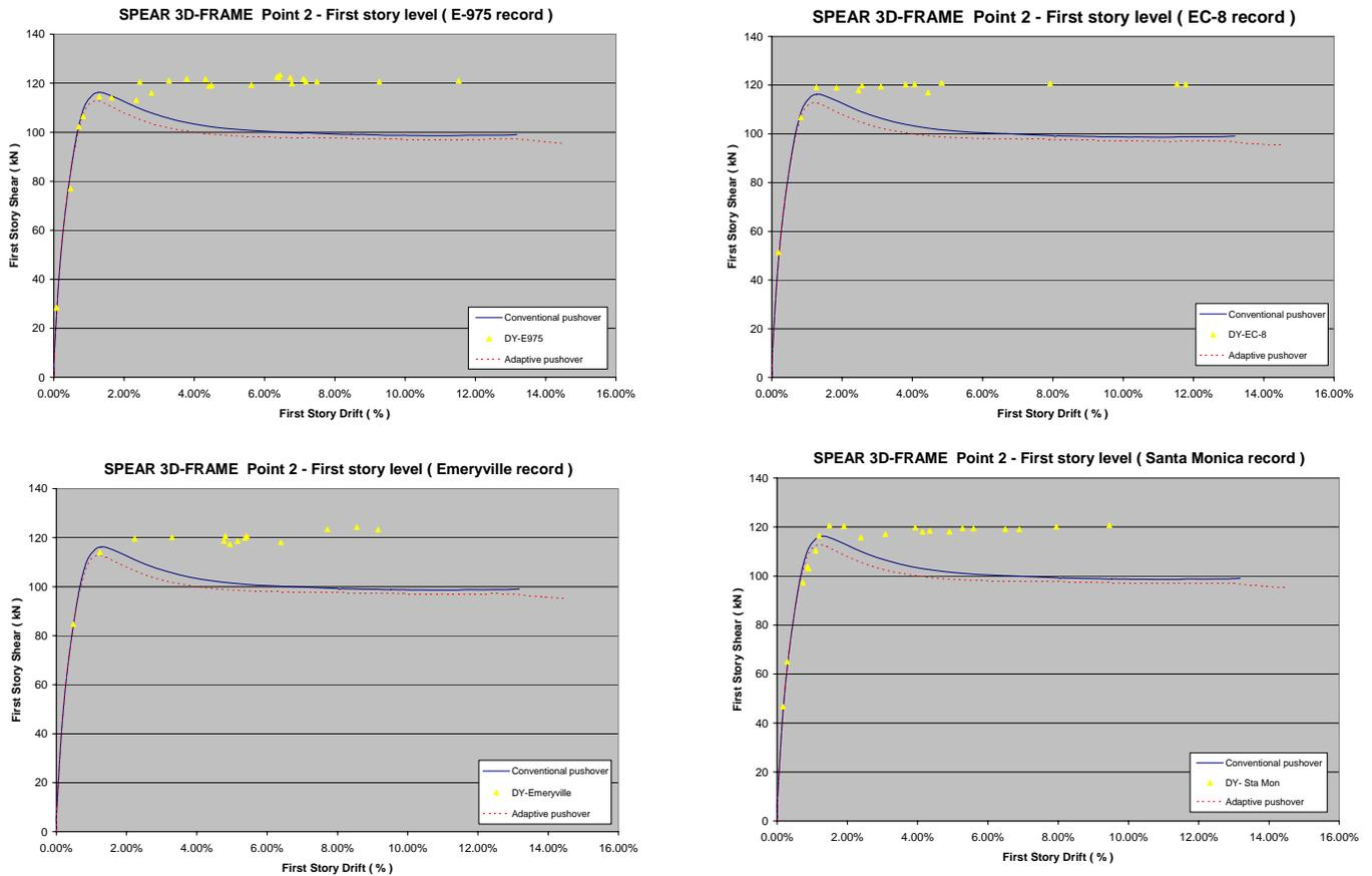
Figure 4.39 Response at the first story level, SPEAR-3D frame
