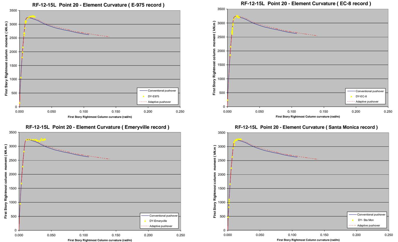
Figure 4.8 Response at the section level, regular structure ( low ductility )
