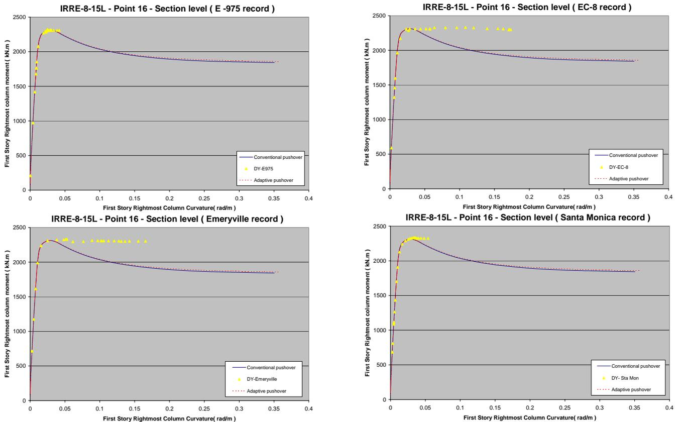
Figure 4.30 Response at the section level, irregular structure ( low ductility )
