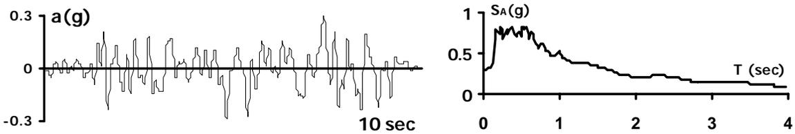
Figure 3.11 Scaled accelerogram response spectrum of the EC-8 record
