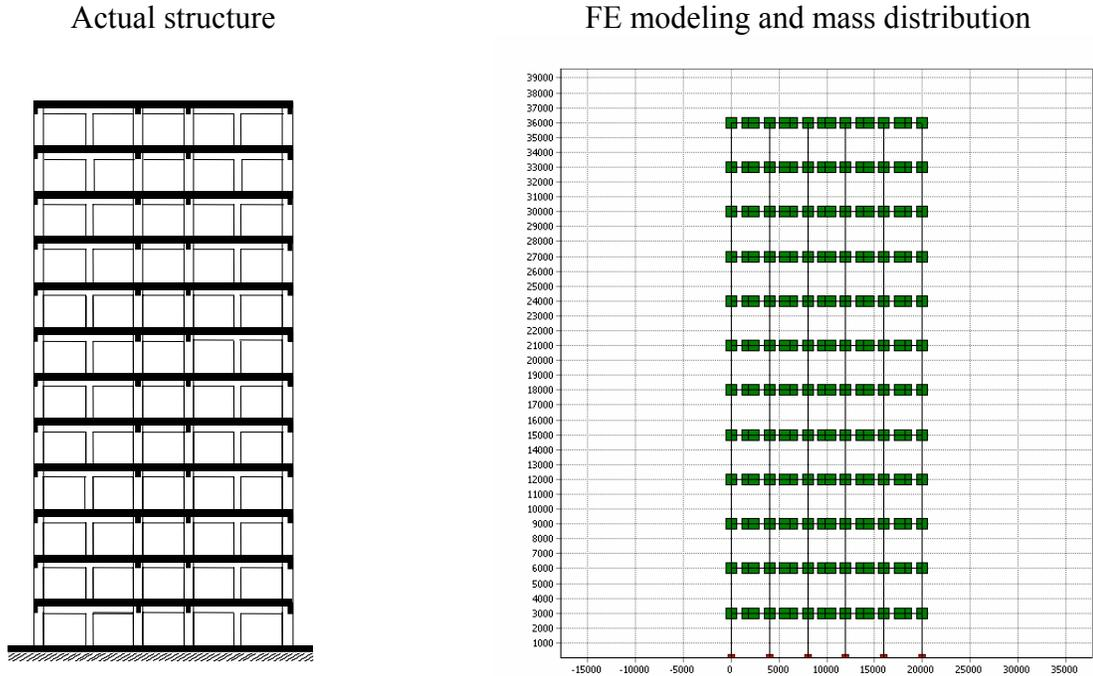
2D reinforced concrete frame
