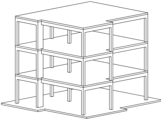
3D reinforced concrete frame
