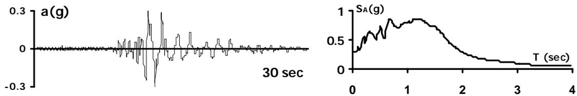
Figure 3.12 Scaled accelerogram and response spectrum of the Emeryville record
