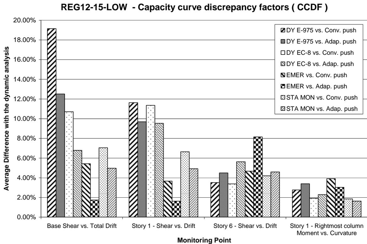
Figure 4.10 Results summary, regular structure ( low ductility )
