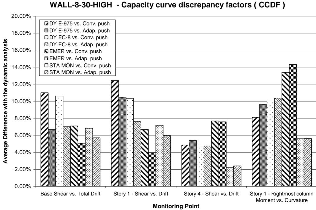
Figure 4.20 Results summary, frame-wall structure ( high ductility )
