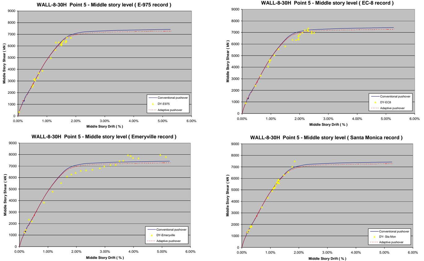
Figure 4.15 Response at the middle story level, frame-wall structure ( high ductility )
