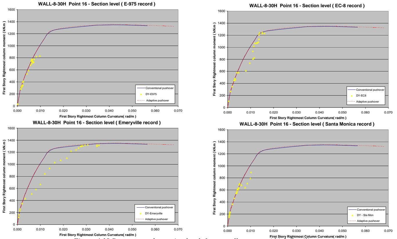
Figure 4.18 Response at the section level, frame-wall structure ( high ductility )
