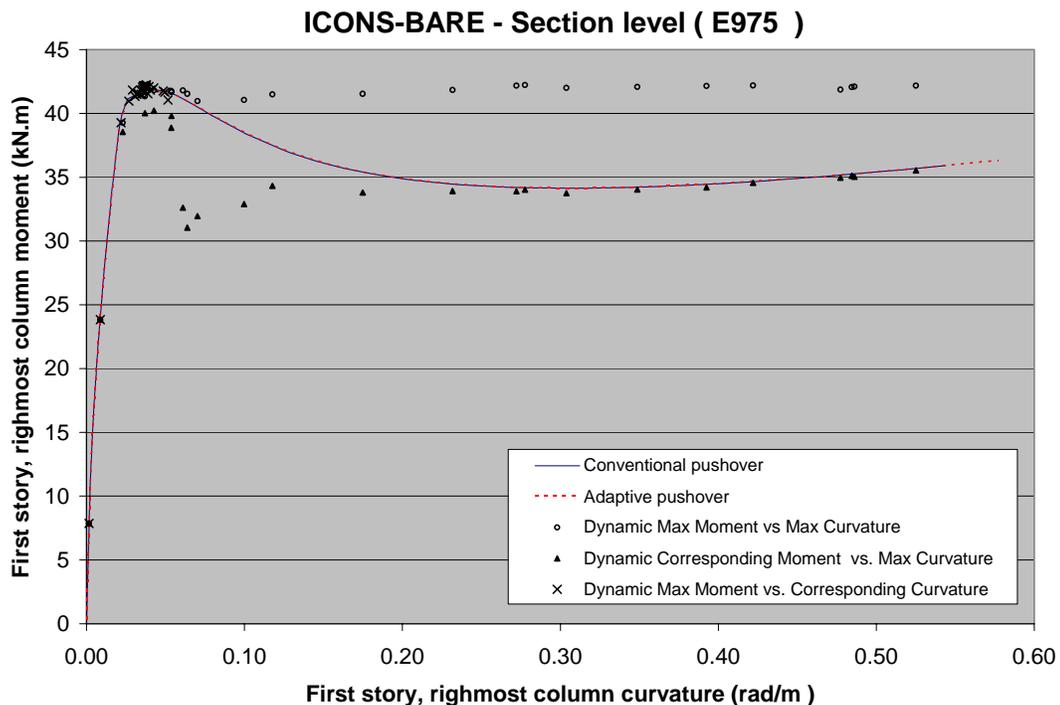
Figure 5.5 Comparison between several methodologies to plot the dynamic analyses results
