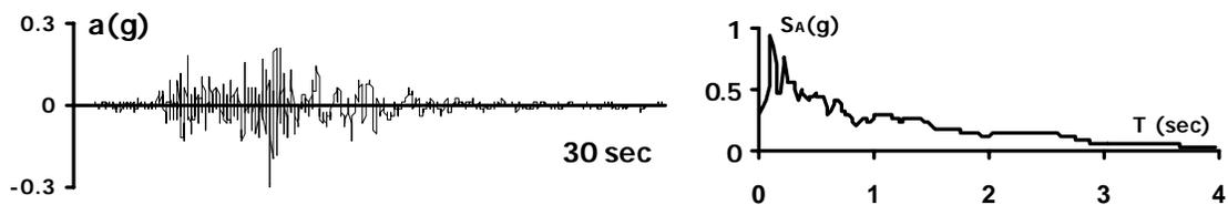
Figure 3.13 Scaled accelerogram and response spectrum of the Santa Monica record
