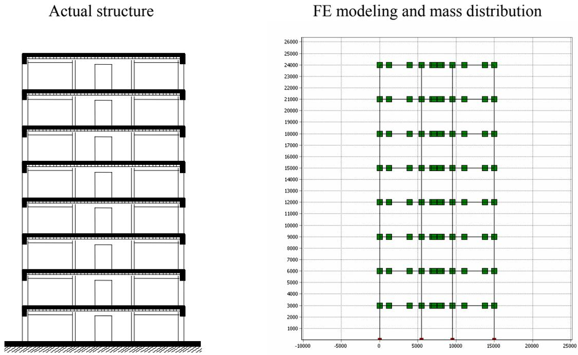
2D reinforced concrete frame
