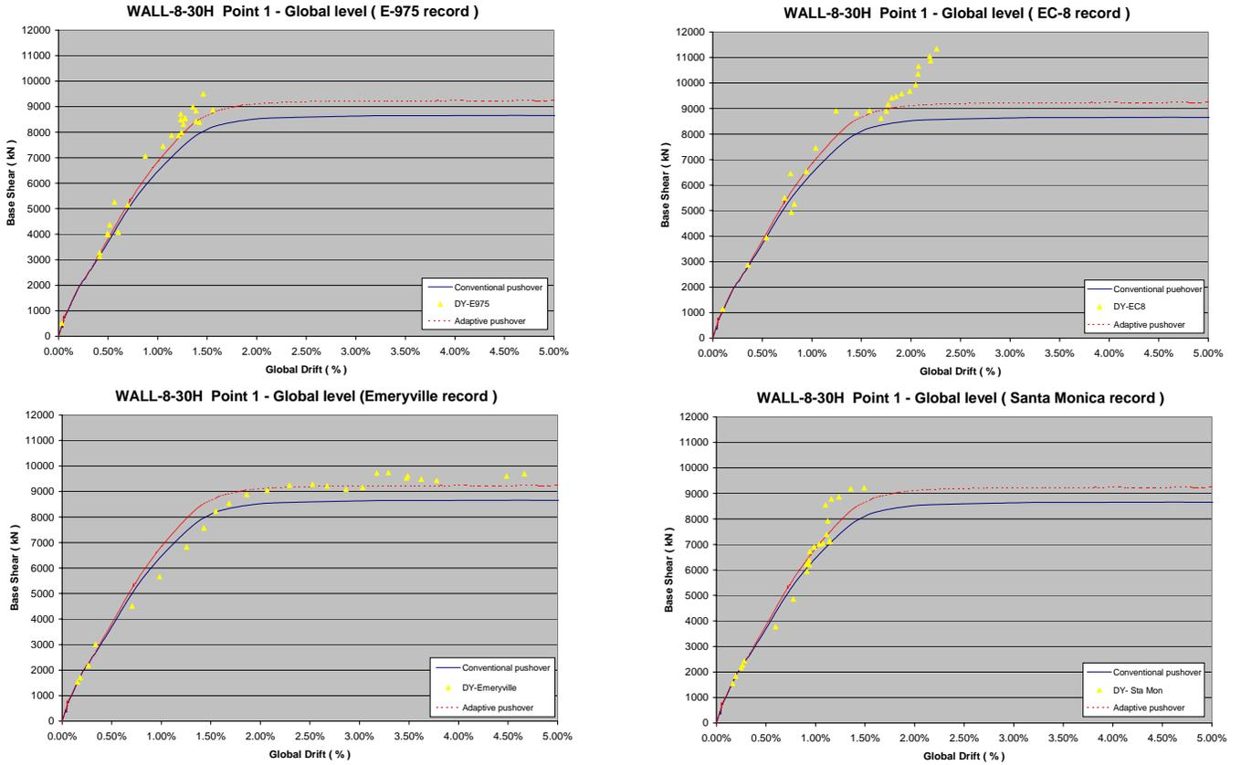
Figure 4.11 Response at the global level, frame-wall structure ( high ductility )
