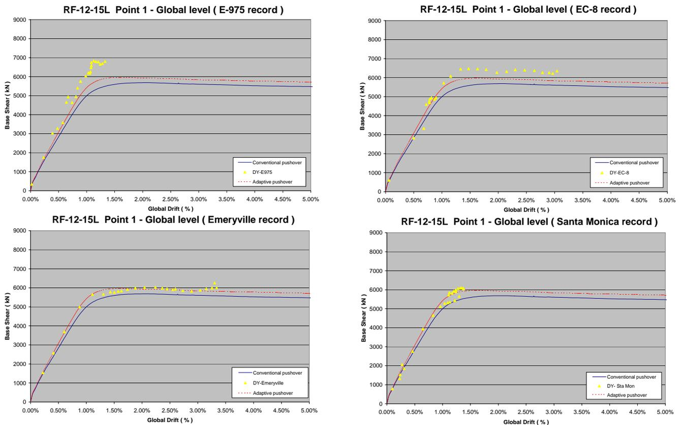
Figure 4.2 Response at the global level, regular structure ( low ductility )
