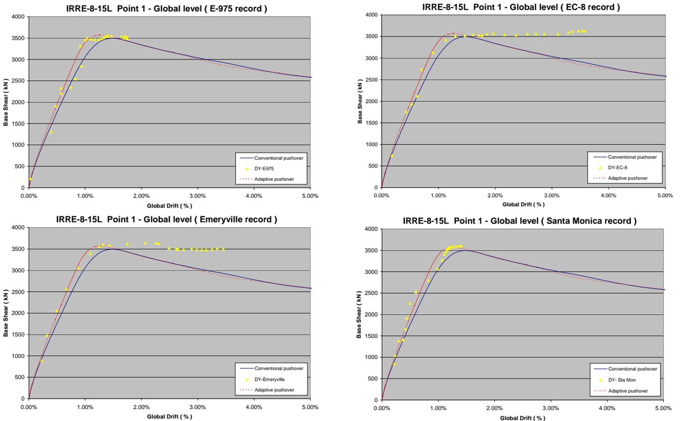
Figure 4.23 Response at the global level, irregular structure (low ductility )
