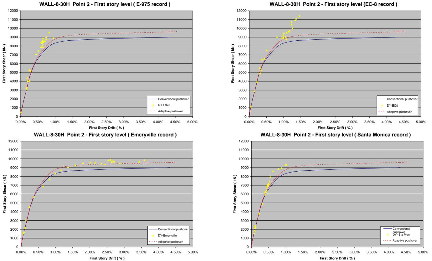
Figure 4.13 Response at the first story level, frame-wall structure ( high ductility )
