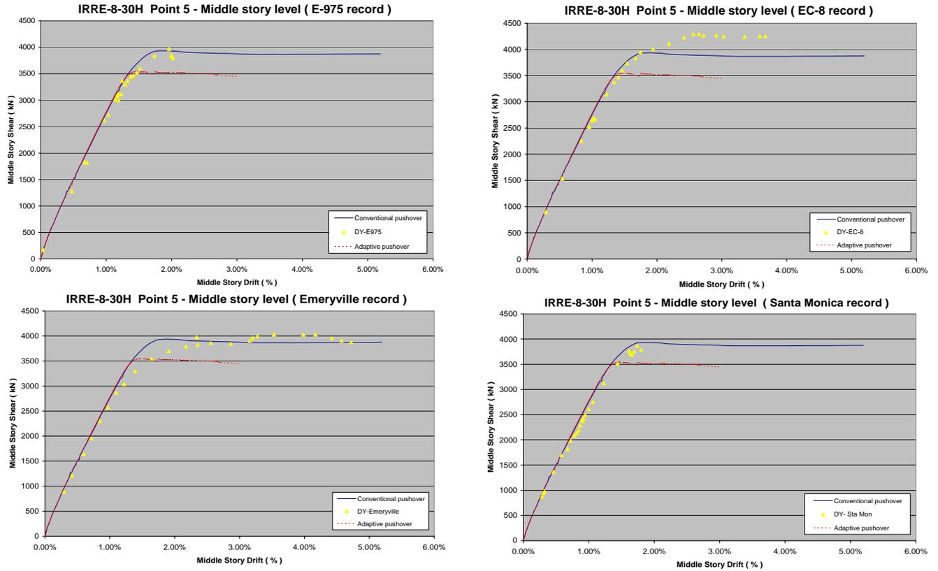
Figure 4.26 Response at the middle story level, irregular structure ( high ductility )
