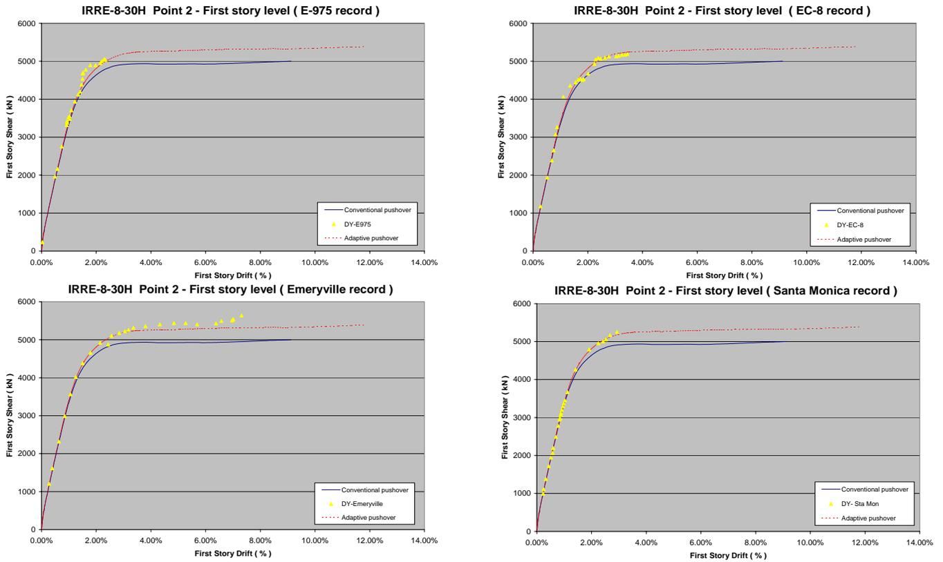
Figure 4.24 Response at the first story level, irregular structure ( high ductility )
