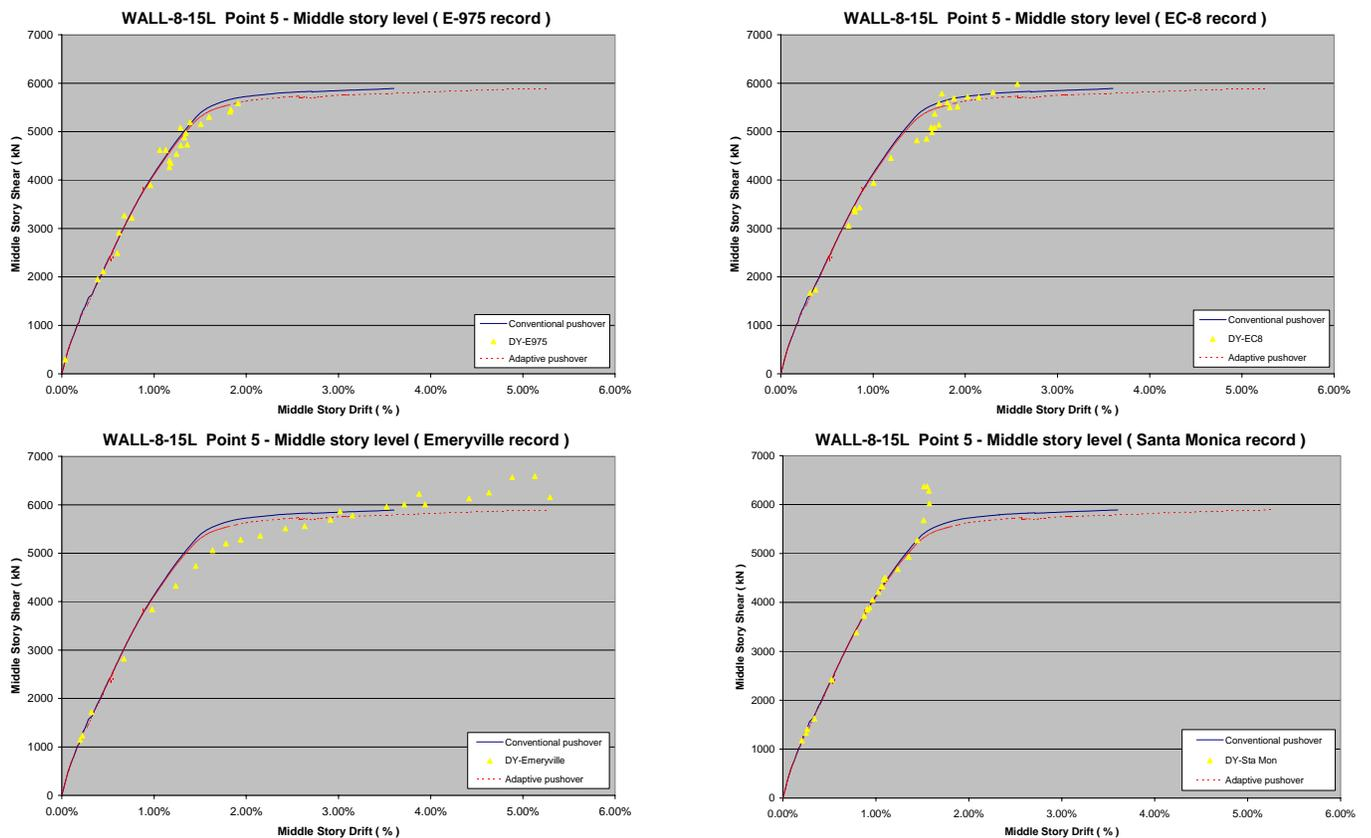
Figure 4.16 Response at the middle story level, frame-wall structure ( low ductility ).
