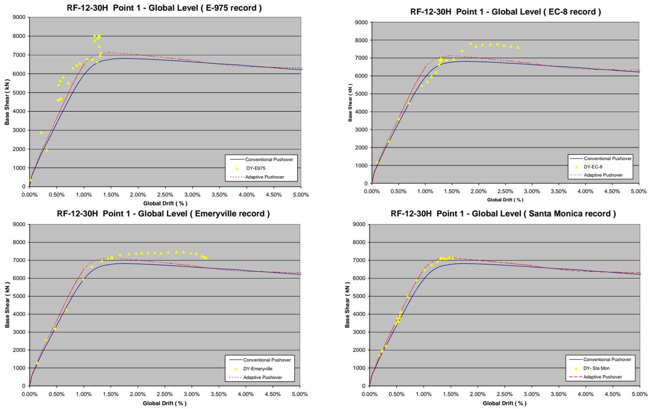
Figure 4.1 Response at the global level, regular structure ( high ductility )
