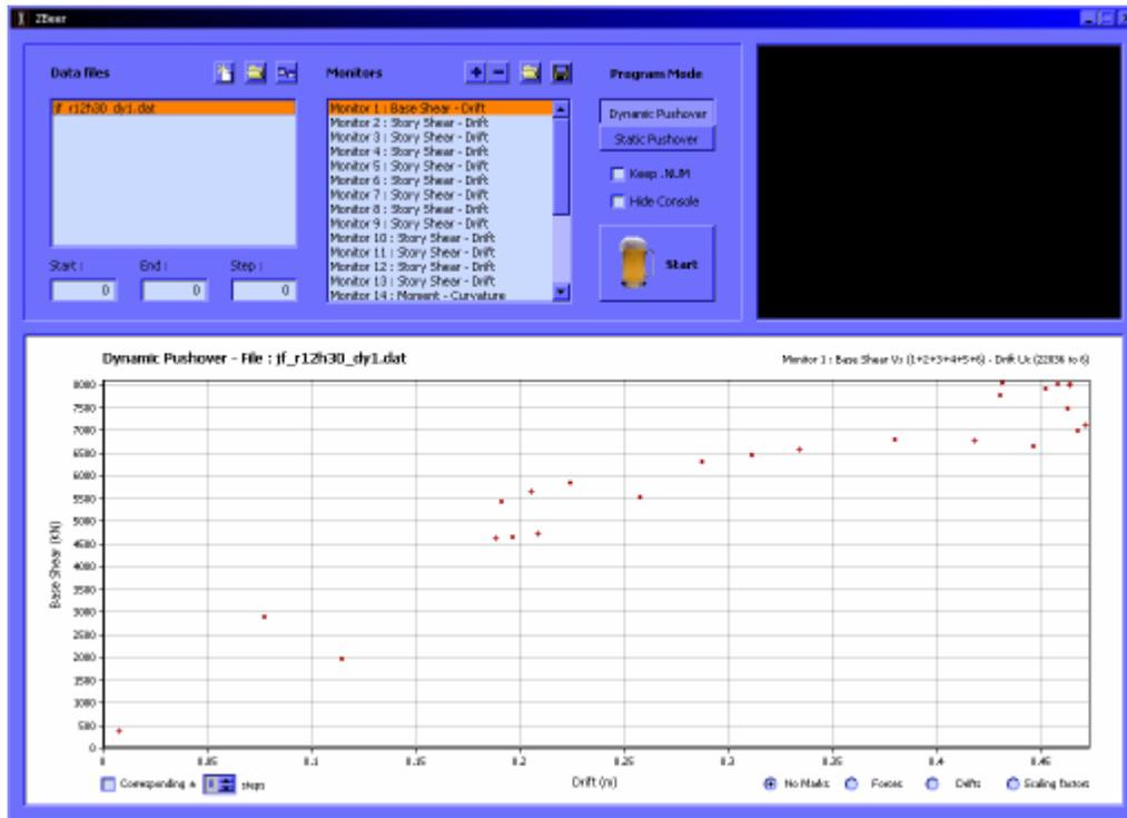
Figure 3.9 Utility developed for IDA generation
