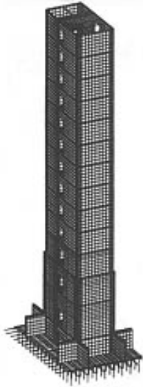
Figure 26. Shell and solid non-linear F.E. model of core and foundation
