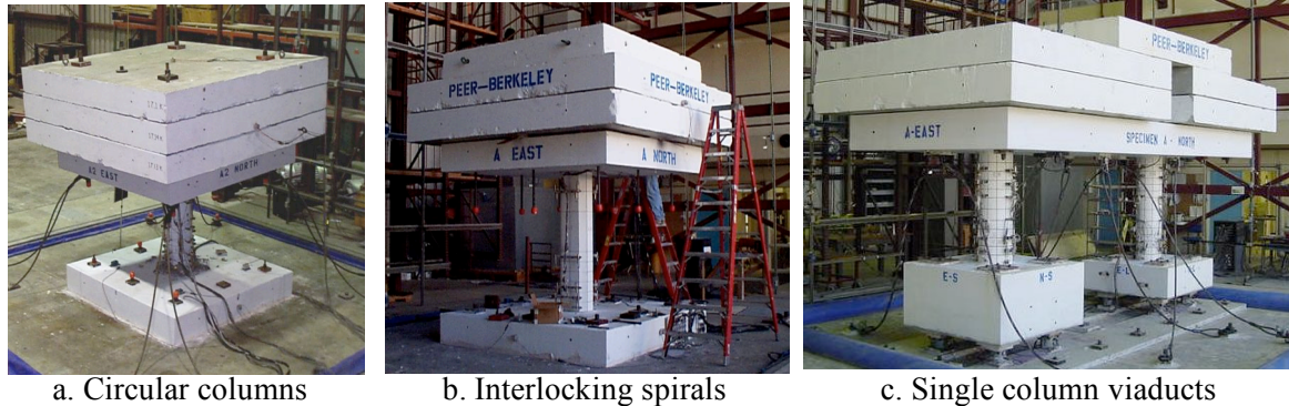
Fig. 1 Recent UC Berkeley shaking table tests of bridge columns
