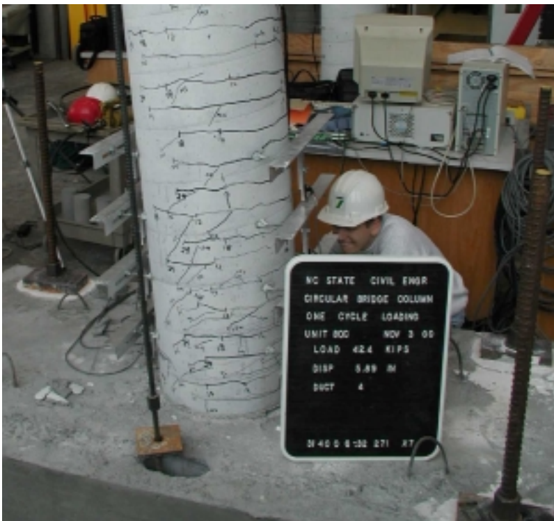
Figure 10.9 East Side of Specimen at Ductility 4
