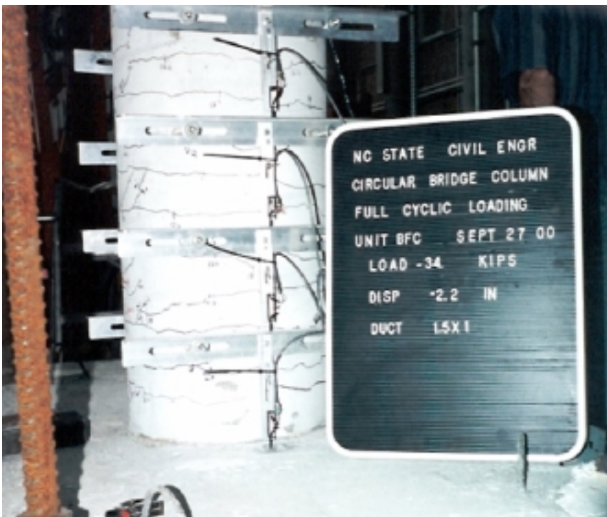
Figure 8.5 North Side of Specimen at Ductility 1.5 Cycle 1
