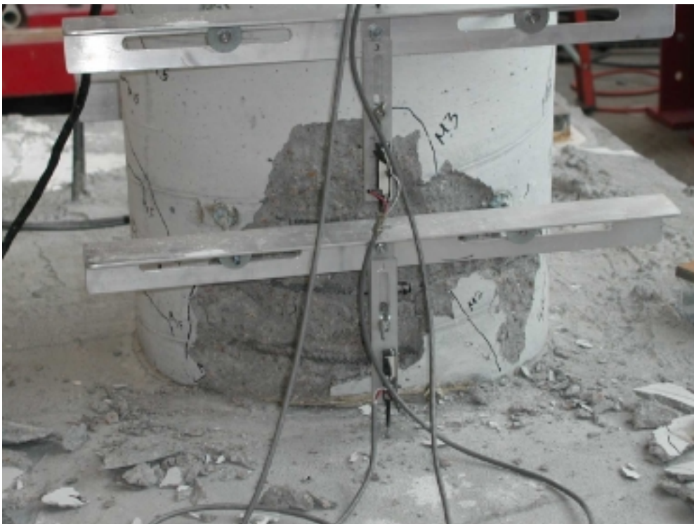
Figure 10.11 South Side of Specimen at Ductility 5
