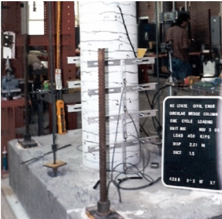
Figure 10.5 North Side of Specimen at Ductility 1.5
