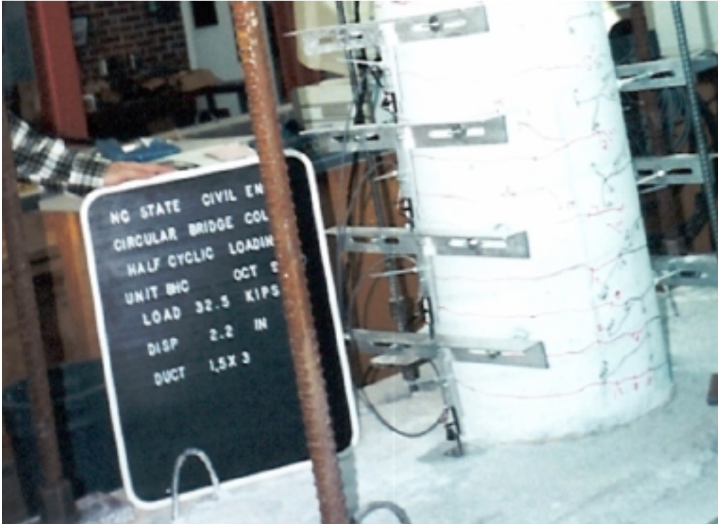
Figure 9.5 South Side of Specimen at Ductility 1.5 Cycle 3
