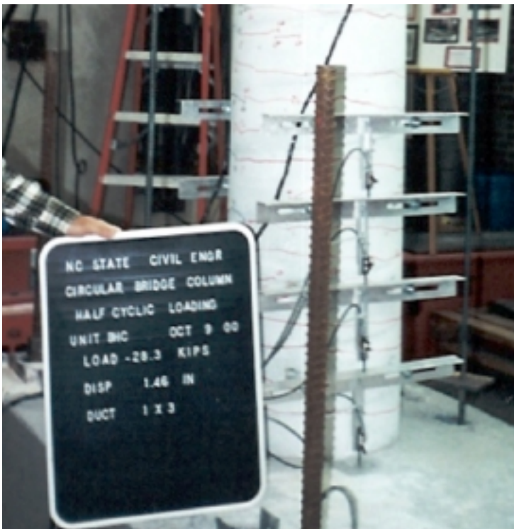
Figure 9.4 South Side of Specimen at Ductility 1 Cycle 3
