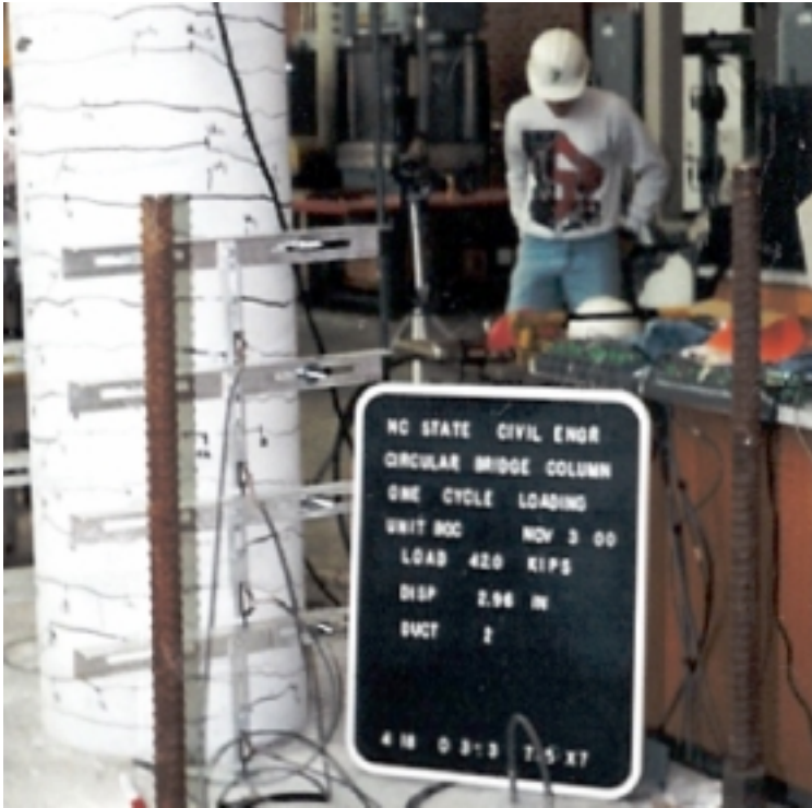
Figure 10.6 North Side of Specimen at Ductility 2
