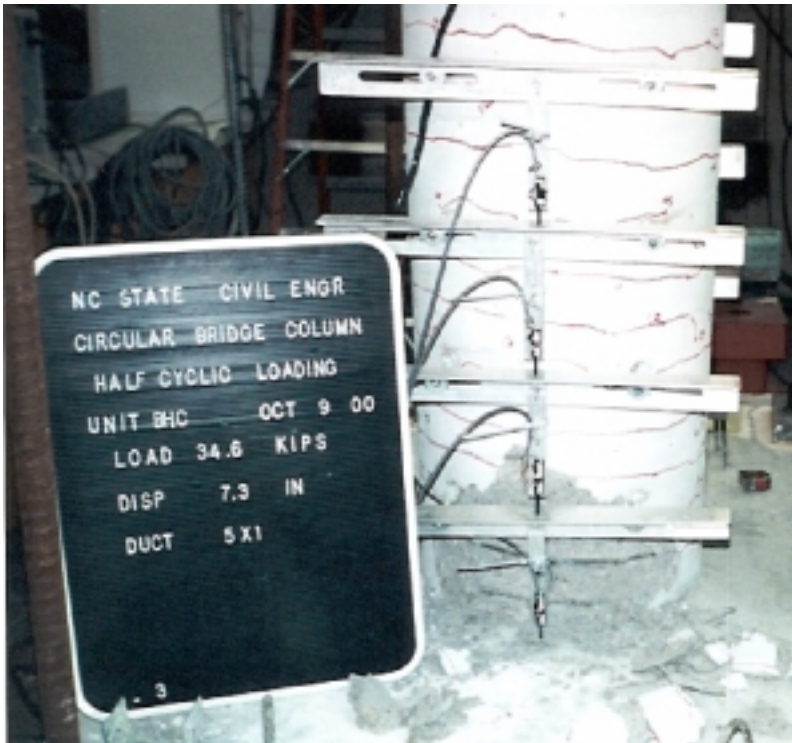
Figure 9.9 South Side of Specimen at Ductility 5 Cycle 1
