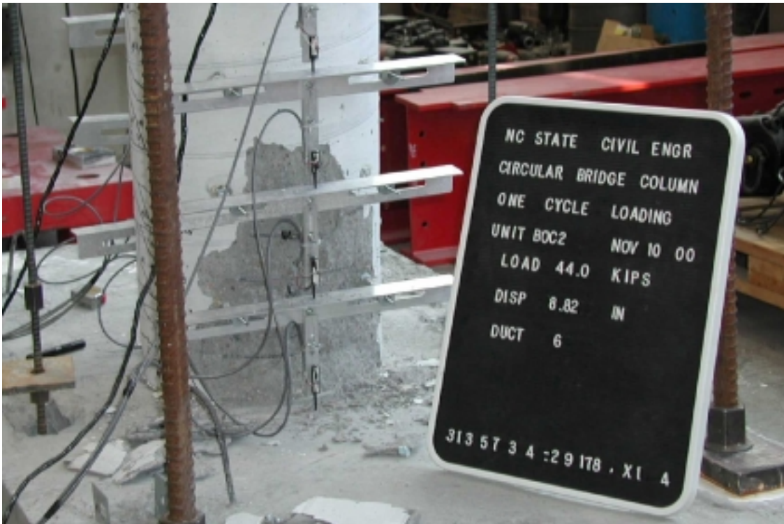
Figure 11.10 South Side of Specimen at Ductility 6
