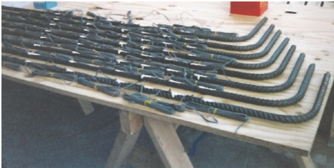
Figure 6.2 Picture of Longitudinal Strain Gages
