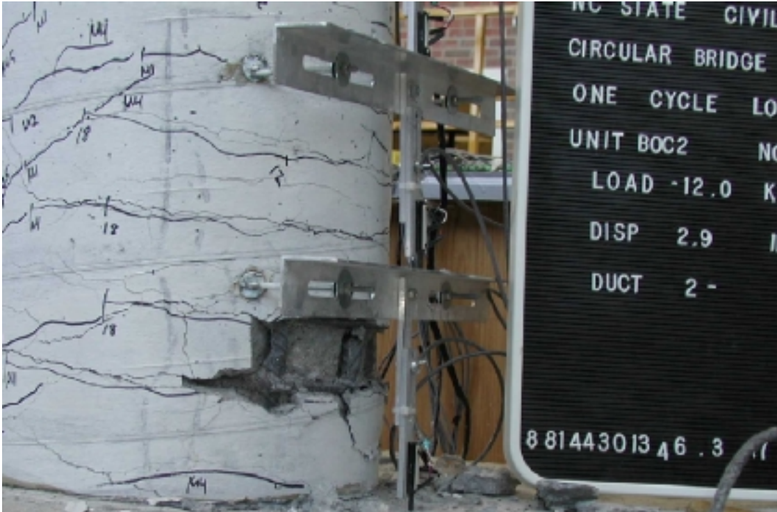
Figure 11.14 North Side of Specimen at 2.9 inches
