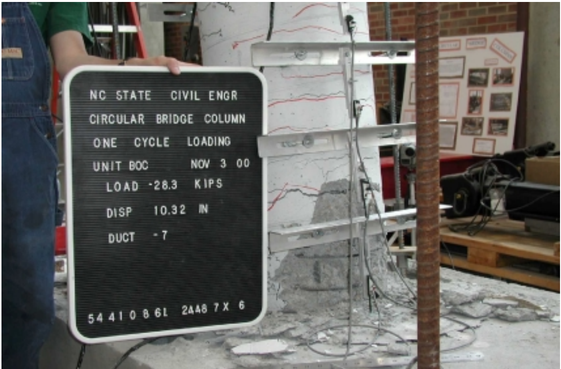
Figure 10.16 South Side of Specimen at Ductility 7 (in the pull direction)
