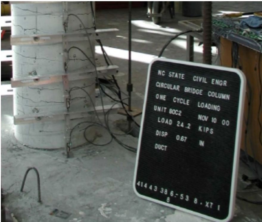
Figure 11.3 North Side of Specimen at Yield
