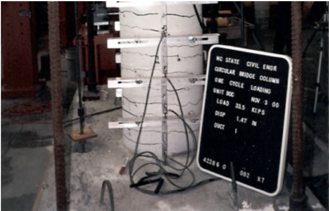
Figure 10.4 North Side of Specimen at Ductility 1
