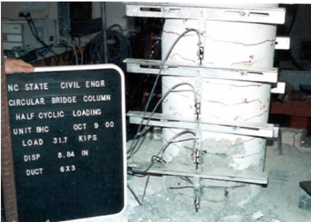
Figure 9.10 South Side of Specimen at Ductility 6 Cycle 3
