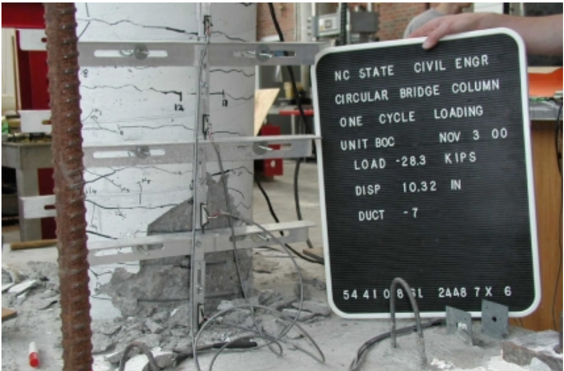
Figure 10.15 North Side of Specimen at Ductility 7 (in the pull direction)
