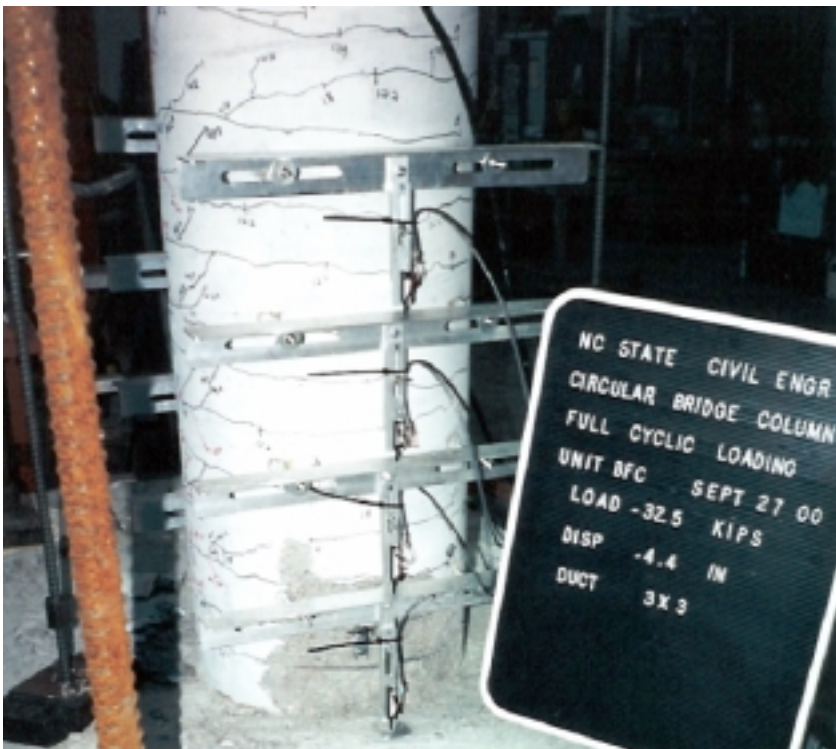
Figure 8.7 North Side of Specimen at Ductility 3 Cycle 3
