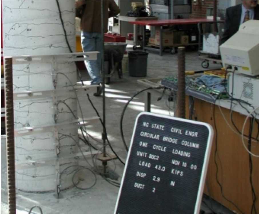
Figure 11.6 North Side of Specimen at Ductility 2
