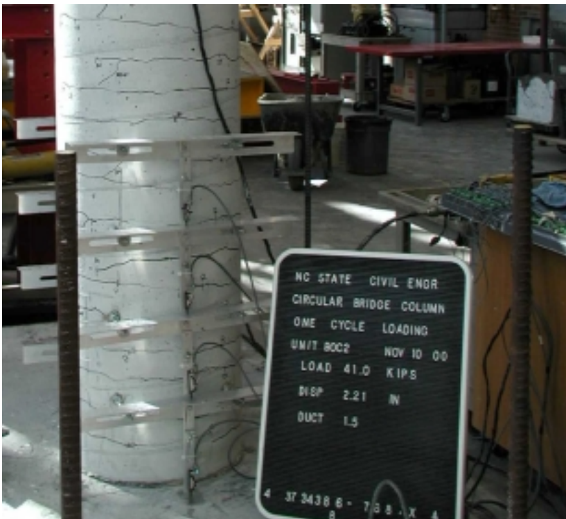
Figure 11.5 North Side of Specimen at Ductility 1.5
