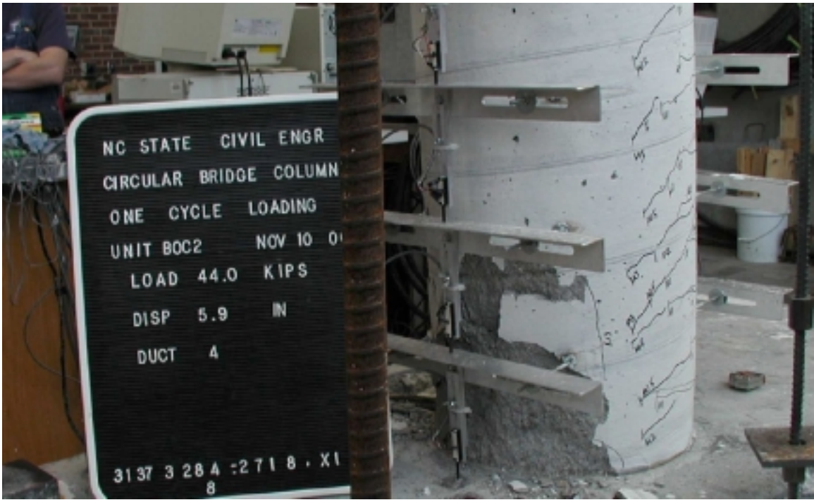
Figure 11.8 South Side of Specimen at Ductility 4
