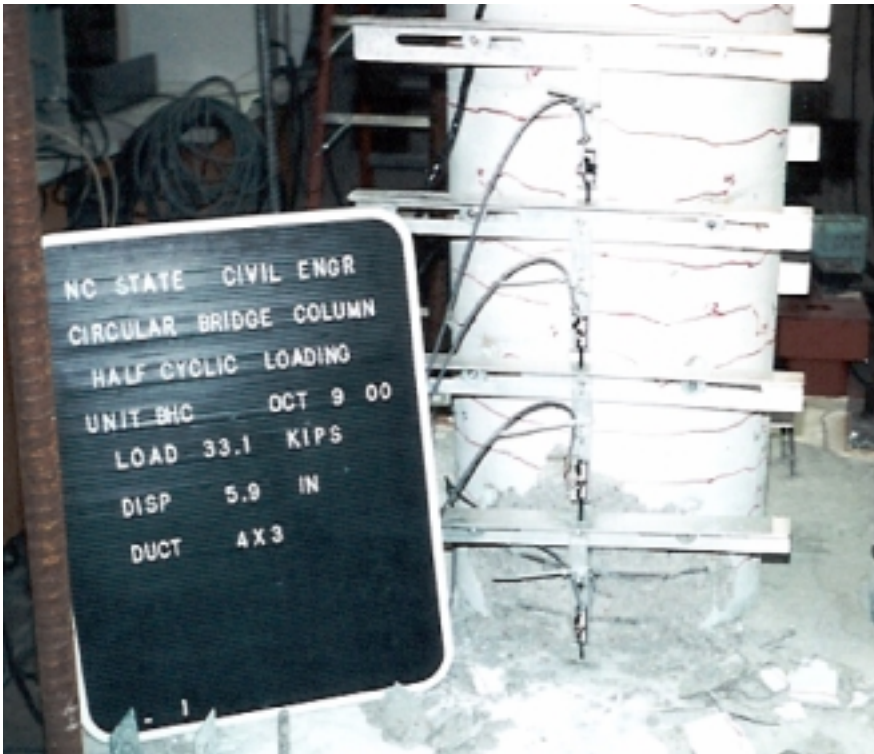
Figure 9.8 South Side of Specimen at Ductility 4 Cycle 3
