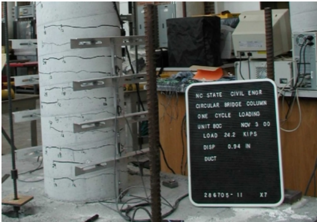
Figure 10.3 North Side of Specimen at Yield
