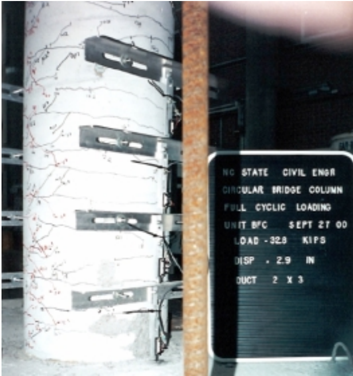
Figure 8.6 North Side of Specimen at Ductility 2 Cycle 3
