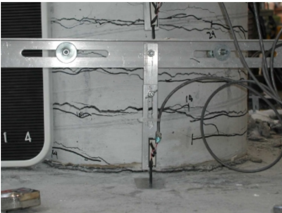
Figure 11.11 North Side of Specimen at Ductility 7
