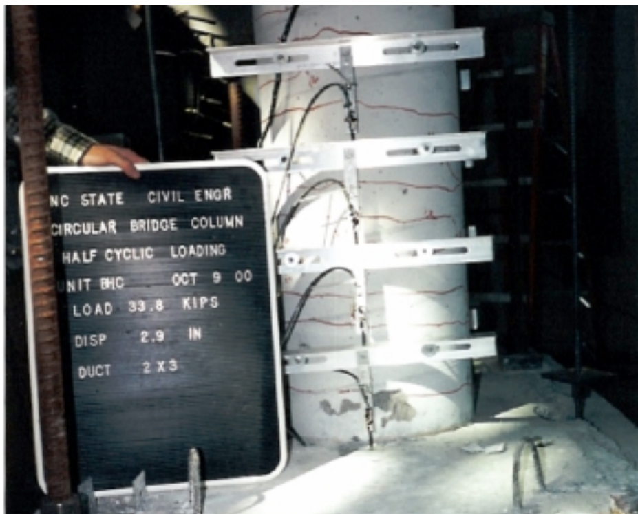
Figure 9.6 South Side of Specimen at Ductility 2 Cycle 3
