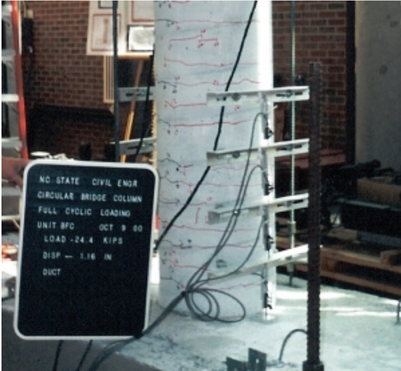
Figure 9.3 South Side of Specimen at Yield
