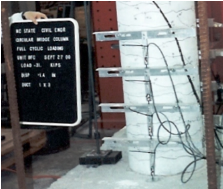
Figure 8.4 North Side of Specimen at Ductility 1 Cycle 3
