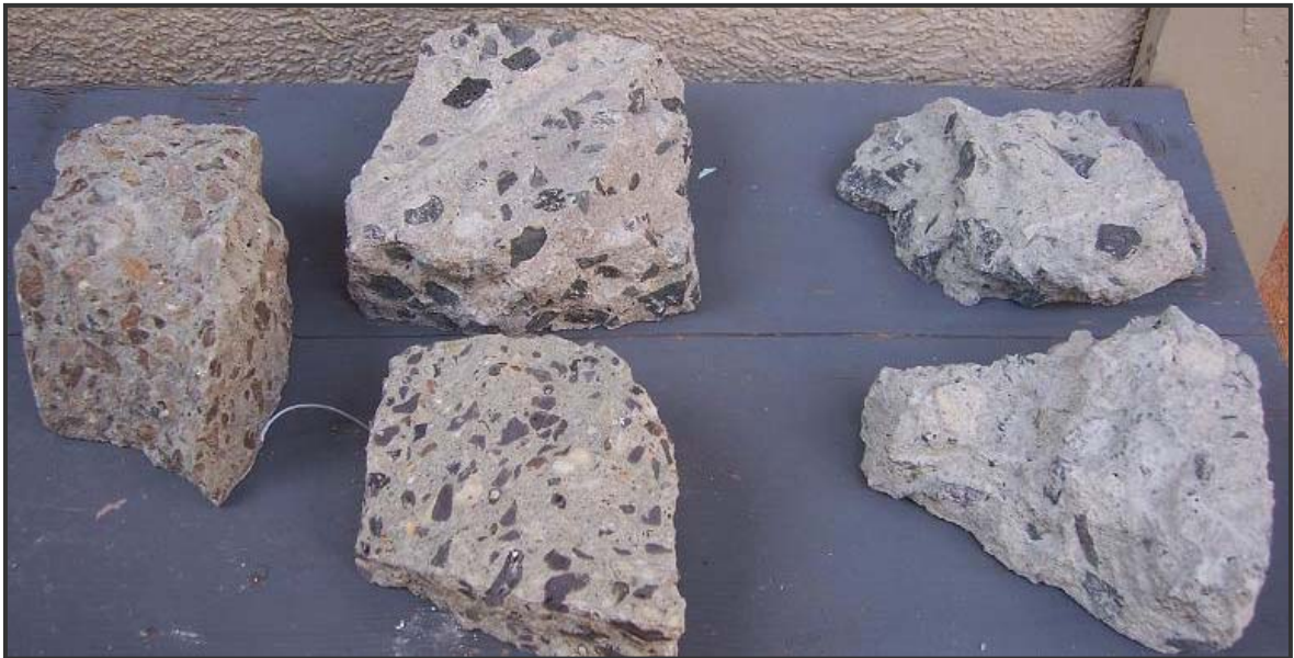
Figure 1.2. Lightweight concrete cracked surfaces (Left) - Normal weight concrete (Right)
