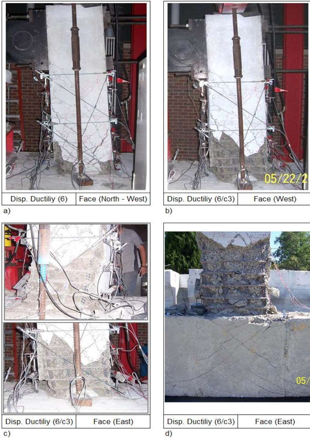
Figure 6.15. Displacement Controlled Loading – (LW2-NS-DSF) – Ductility Six to Failure
