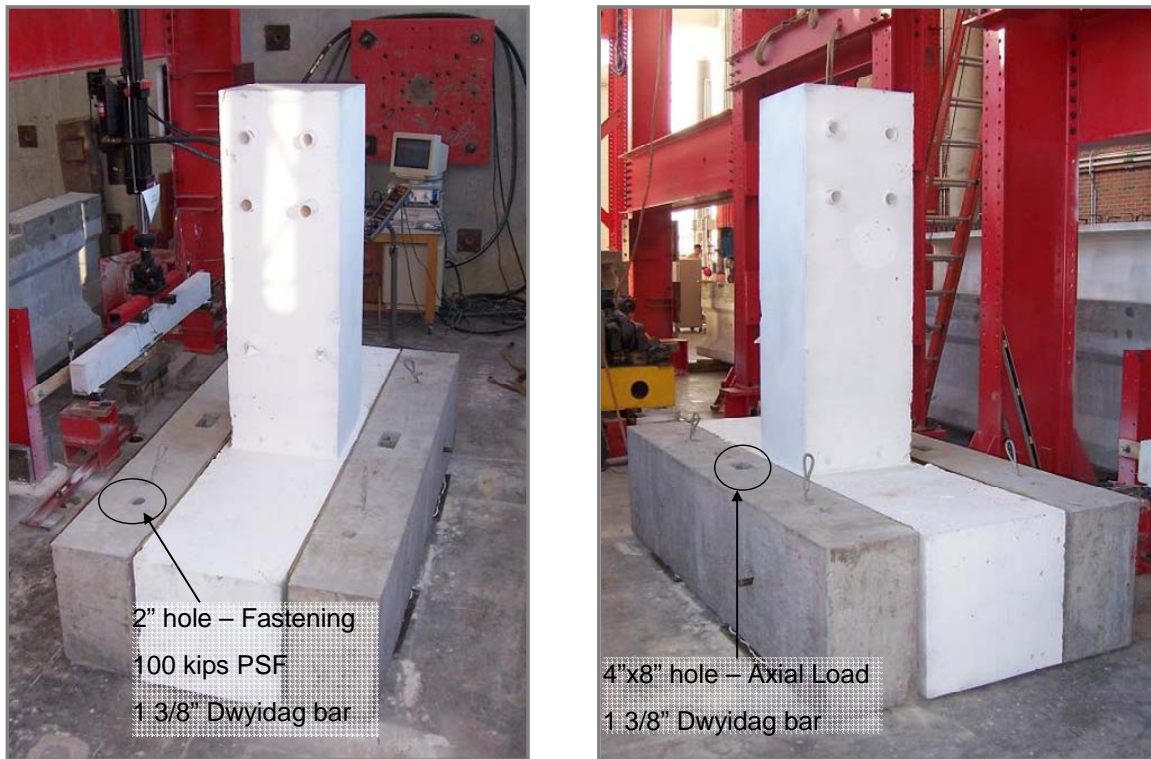
Figure 4.5. Fastening Ducts Locations
