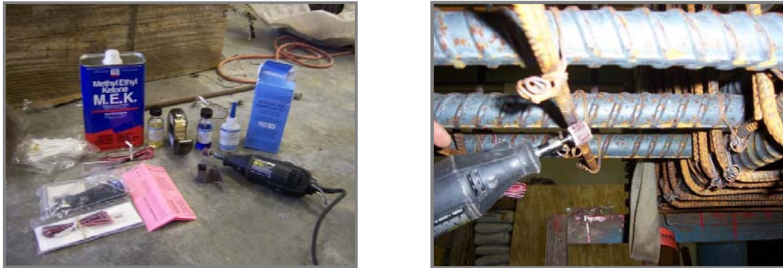
Figure 4.8. Strain Gages Setup – Materials Used (Left), Grinder (Right)
