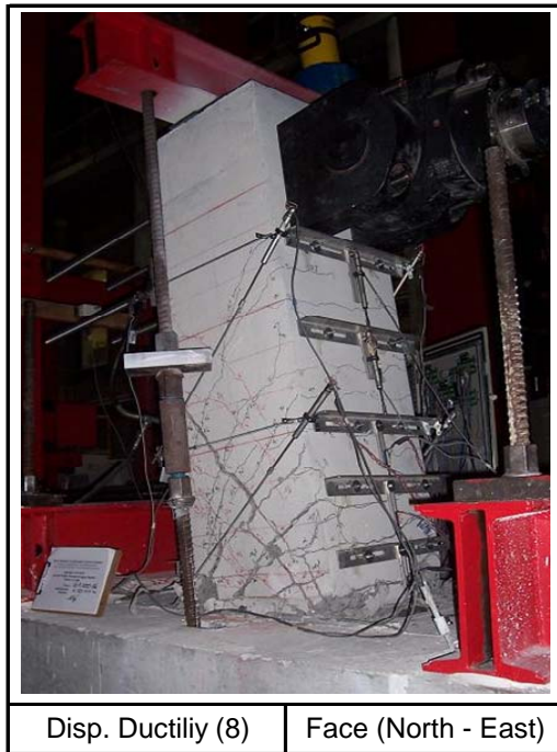
Figure 6.5. Displacement Controlled Loading – (NW-NS-DSF) – Ductility Six to Failure
