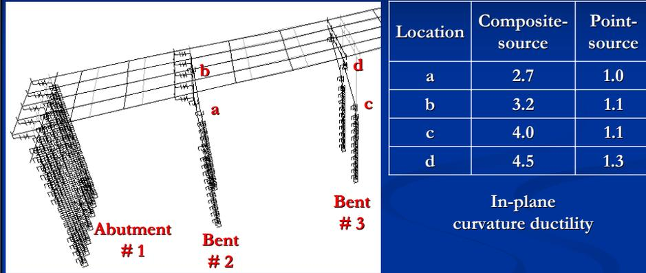
Motions applied along the **transverse axis** of the bridge
