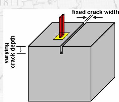
Cement-past cube with a notch cut using hacksaw to generate a crack of varying depth.
