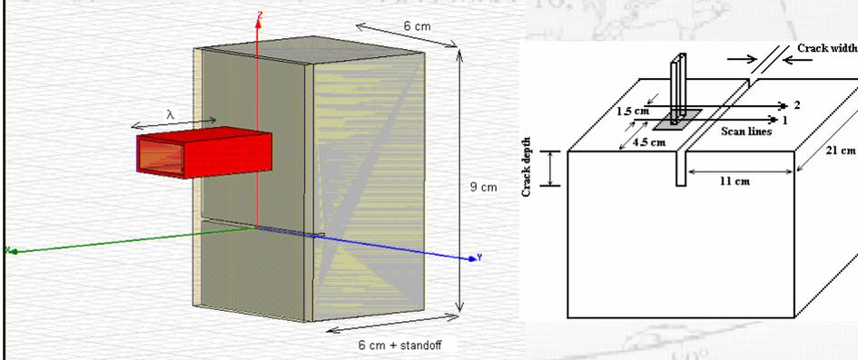
Schematic of HFSS model developed for simulating crack characteristic signals (CCS).
