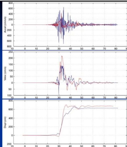
Observed (red) vs. synthetic (blue) ground motions at station T052 (NS component) during 1999 Chi-Chi earthquake (reverse)
