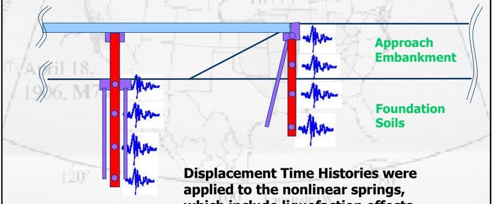
Displacement Time Histories were applied to the nonlinear springs, which include liquefaction effects
