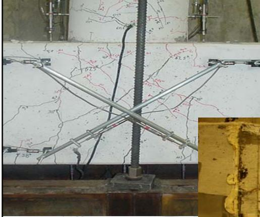
Excessive cracks of unretrofitted specimen
