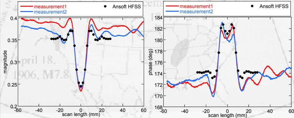
Magnitude and phase of measured and simulated crack characteristic signals for a crack of 1.14 mm wide, 5.0 mm deep, at a standoff distance of 1.0 mm and for a dielectric property of  $(5.96 - j1.02)$  at 10.0 GHz using *Arrangement 2*.
