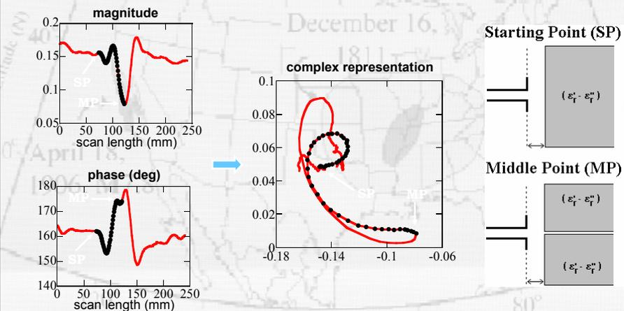
Complex plane representation of reflection coefficient of 2 mm-wide crack at a standoff distance of 2.0 mm on day 13.
