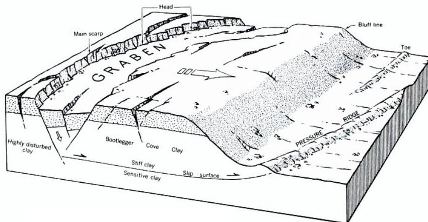
Block diagram of a lateral spread which evolved from post-1964 earthquake evaluations in Alaska by Walt Hansen in USGS Professional Paper 542-A (1966)
