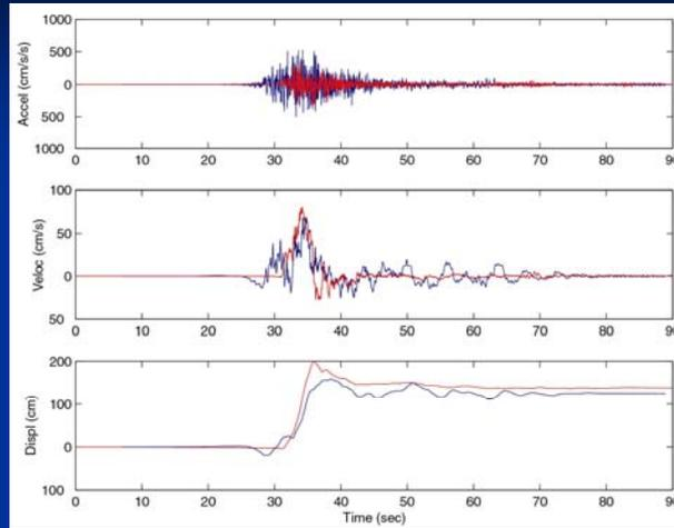
Observed (red) vs. synthetic (blue) ground motions at station SKR (east horizontal component) during 1999 Kocaeli earthquake (strike-slip)
