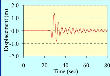
Sim #82 – FN ground motion with displacement pulses
