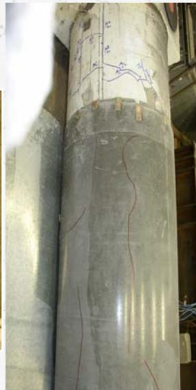
Plastic hinge formed at the beam-column joint of the retrofitted specimen
