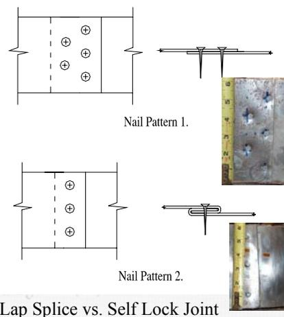
Lap Splice vs. Self Lock Joint
