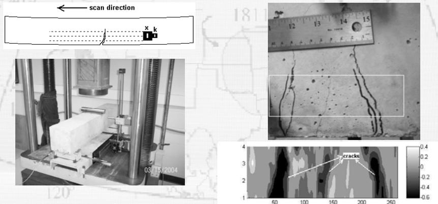
4 lines with 125 mm of scan length (2 data points/mm shown)
