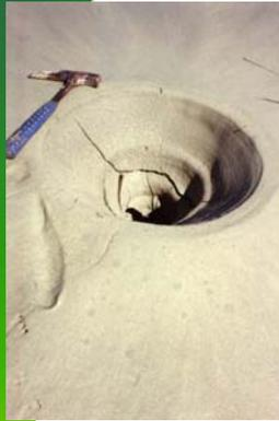
Liquefaction is a failure mechanism by which cohesionless materials lose shear strength when the pore pressure is excited to a level equal to the effective confining stress. Usually limited to the upper 50 feet and typically occurs in silt, sand and fine gravel.
