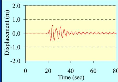
Sim #32 – FN ground motion without displacement pulses
