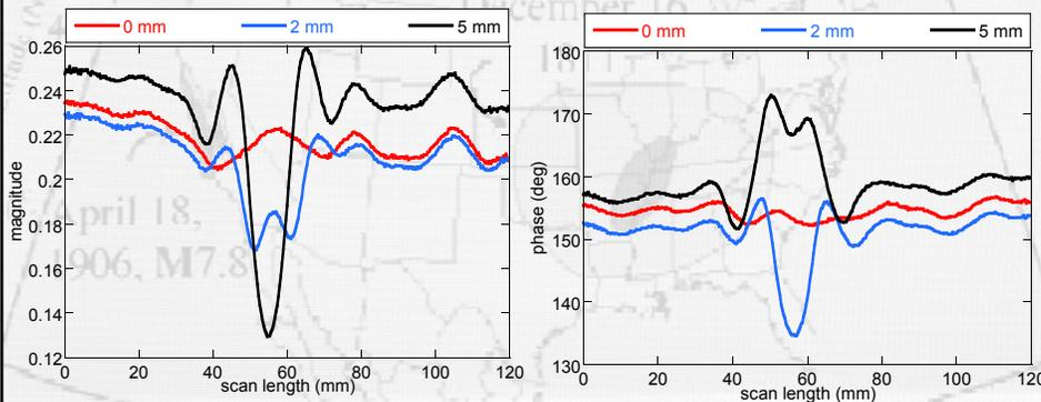
Magnitude and phase of reflection coefficient of a 1.14-mm wide crack for different crack widths at a standoff distance of 2.0 mm (Arrangement 2 @10 GHz).
