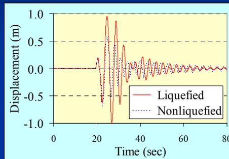
FN at bottom of embankment
