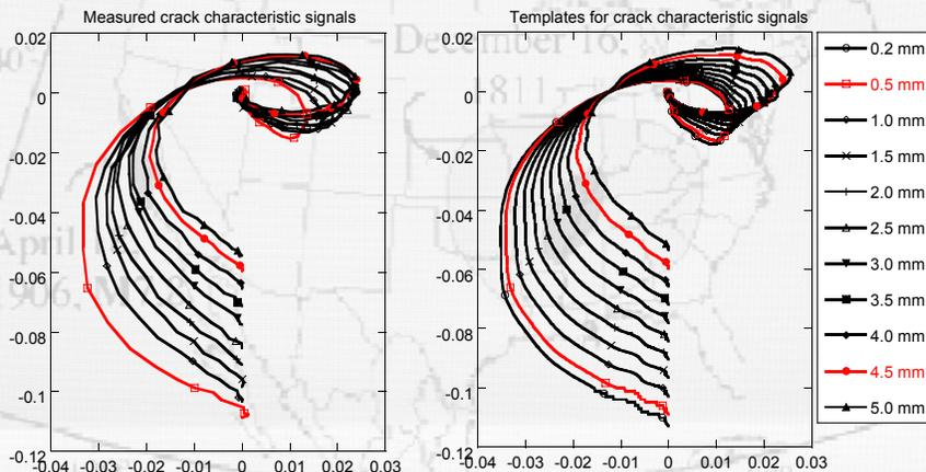
Templates at other standoff distances are obtained by interpolating or extrapolating the measurement signals at standoff distance of 0.5 mm and 4.5 mm
