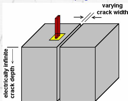
Two mortar cubes used to simulate cracks with varying crack width.
