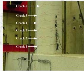
(a) Crack pattern at 177.3 kN
